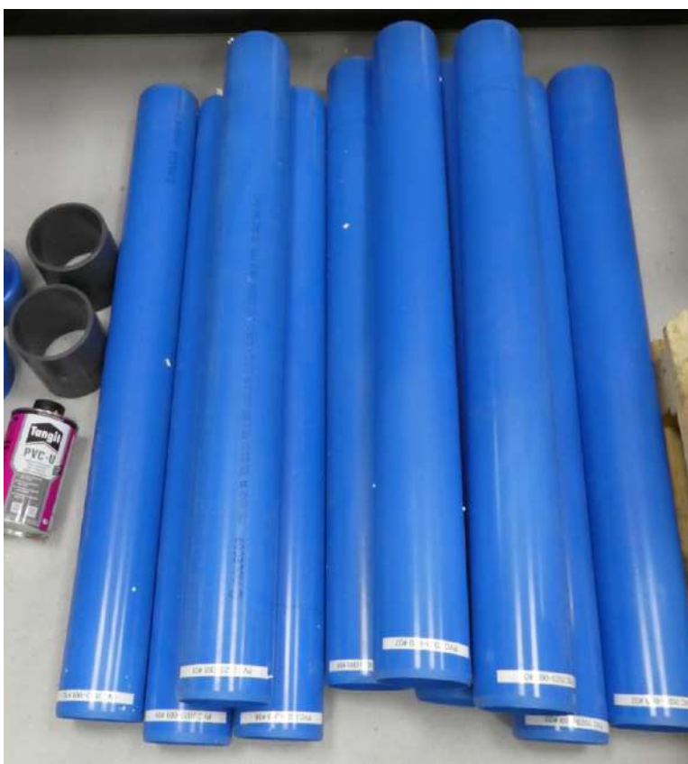
Figure 4: the PVC-O pipes, M-110 (solvent cement couplers) a can of Tangit supplied by Molecor
