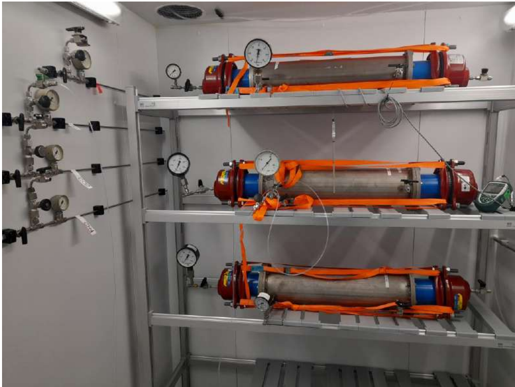
Figure 6: the test setup showing the samples in the temperature controlled test chamber.
