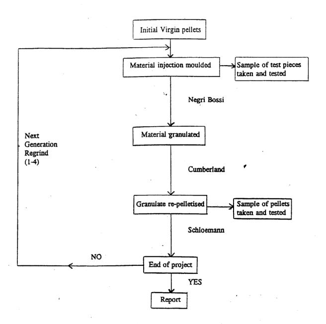
1 pass of material = Injection moulding, granulation, compounding (pelletising).
