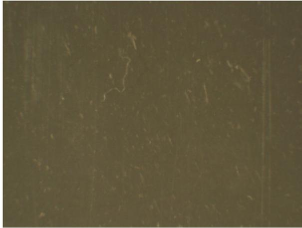
Fig. A.4 Inner wall surface; small damages and craze (shown surface: ca. 10x10 mm).
