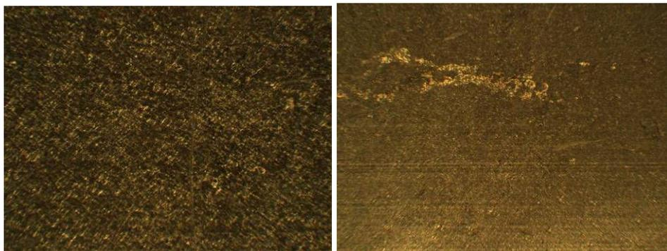
Fig. IV.3 Surface inner pipe wall; remainder of sewage sediment (shown surface right: ca. 10x10 mm; left: magnification 6x right photograph).
