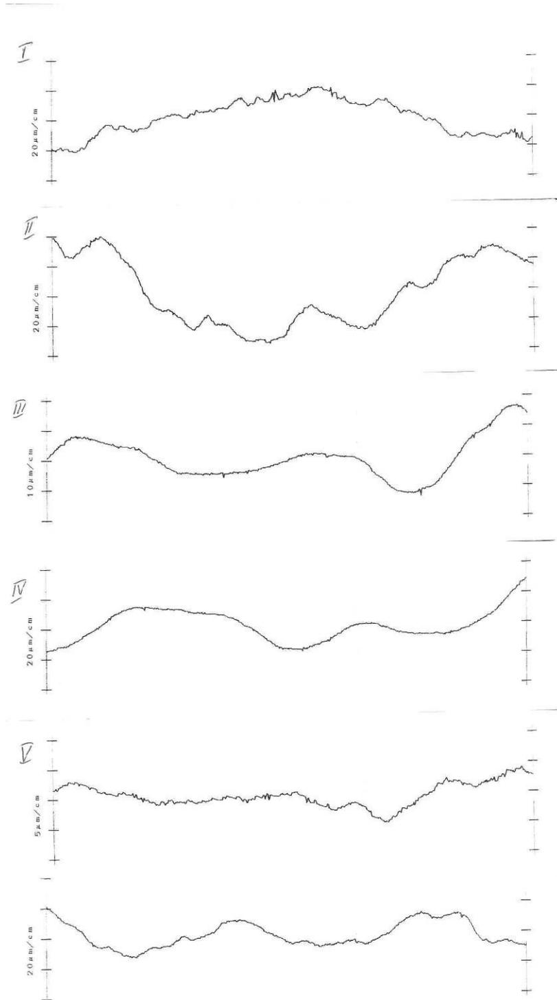
Fig. 2.1 Global surface roughness measurements on soaked and rinsed inner pipe surfaces of the pipes under study (I-VI) measured over 16 mm.
