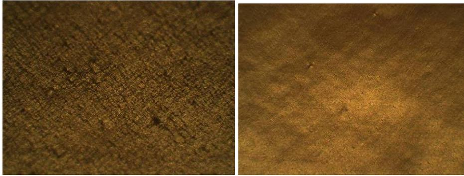
Fig. II.4 Surface inner pipe wall; non-smoothness ascribed to production process (shown surface right: ca. 10x10 mm; left: magnification 6x right photograph).
