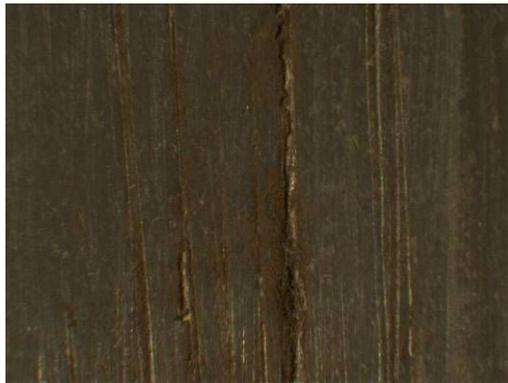
Fig. A.3 Inner wall surface; wear tracks in the length direction of the pipe (shown surface: ca. 10x10 mm).
