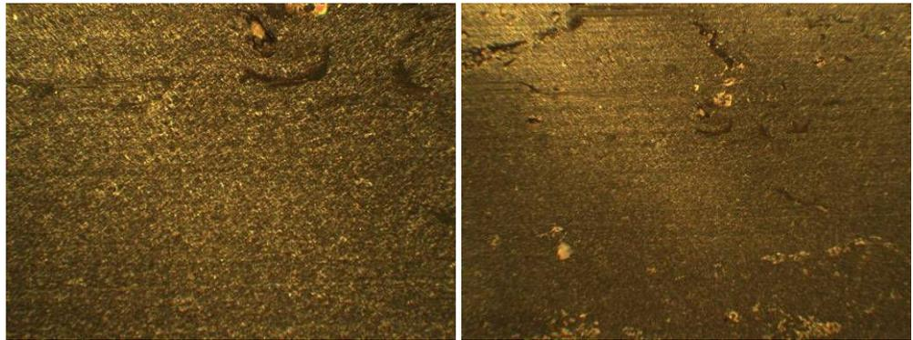
Fig. IV.4 Surface inner pipe wall; remainder of sewage sediment (shown surface right: ca. 10x10 mm; left: magnification 6x right photograph).
