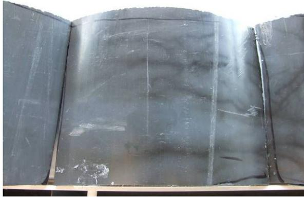
Fig. A.1 Stained pattern on outer pipe wall.
