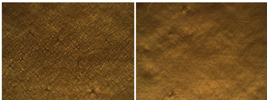
Fig. II.3 Surface inner pipe wall; non-smoothness ascribed to production process (shown surface right: ca. 10x10 mm; left: magnification 6x right photograph).
