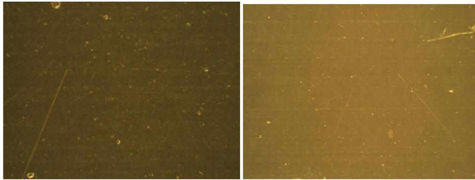
Fig. V.4 Surface inner pipe wall (shown surface right: ca. 10x10 mm; left: magnification 6x right photograph).
