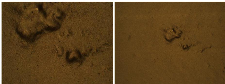
Fig. I.3 Surface inner pipe wall; non-smoothness ascribed to production process (shown surface right: ca. 10x10 mm; left: magnification 6x right photograph).
