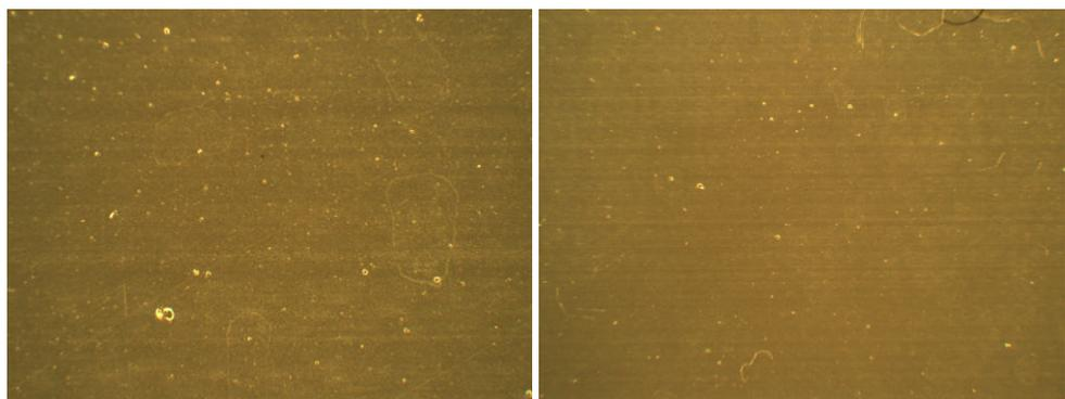
Fig. V.3 Surface inner pipe wall (shown surface right: ca. 10x10 mm; left: magnification 6x right photograph).
