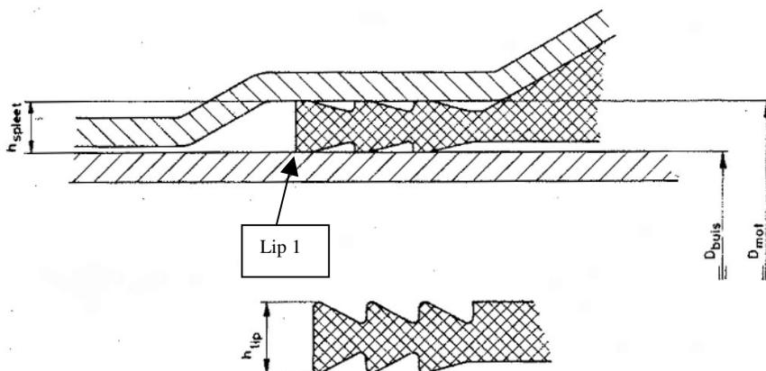
*Figure 2. Detail of socket joint*
