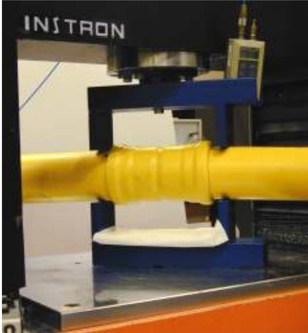
*Fig. 1 Test rig for extreme deflection tests*
