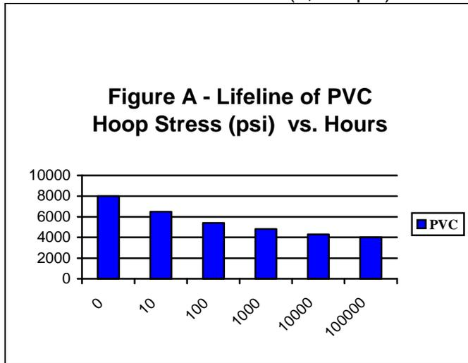
Thus one may ask what would be a suitable maximum tensile strength for long-term pressure pipe applications. It has been determined that the strength of a thermoplastic resin at 100,000 hours can effectively be defined as the long-term strength of the material. This point is defined as the Hydrostatic Design Basis (HDB) of the plastic compound. In this case, for PVC 12454 compound as specified by most pressure pipe standards, the HDB will be 27.6 MPa (4,000 psi).
