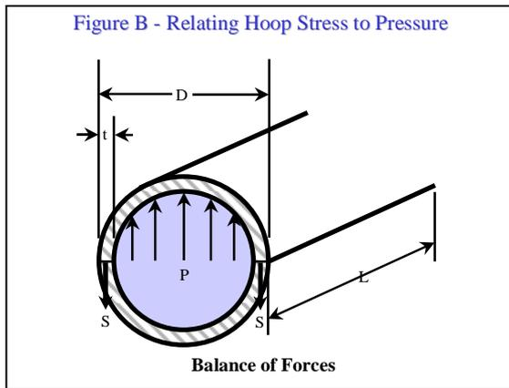
Assuming the stress is acting on the centre of the pipe wall, the balance of forces analysis will yield,  $P (OD - t) = 2 (S)(t)$ , where  $P$  = internal pressure, and  $S$  = resultant hoop stress on the material. By substituting  $DR$  for  $OD/t$ , the equation can be rearranged to be  $P (DR-1) = 2St$ , or  **$P = 2S / (DR-1)$** .
