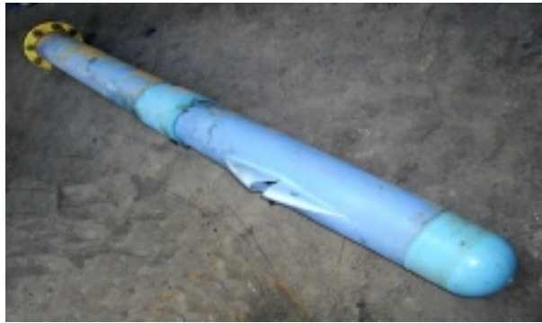
Fig.1. Typical failure mode at elevated pressure
