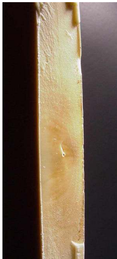
Crack growth starting from inhomogeneity in pipe wall
