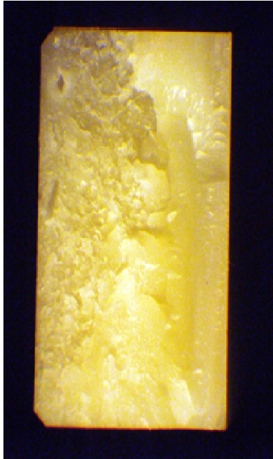
Fractured surface after impact (4x6 mm)
